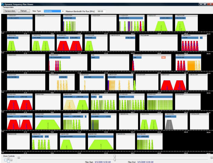
ECM'S DYNAMIC FREQUENCY PLAN VIEWER SHOWS CURRENT SATELLITE LOADING IN REAL-TIME AS WELL AS PAST, AND FUTURE CAPACITY ALLOCATIONS
